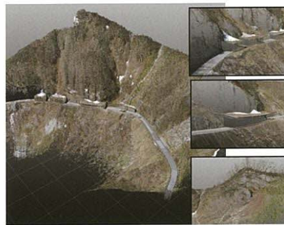
Three-dimensional point cloud data by laser surveying
