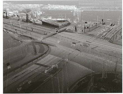
3D point cloud data by MMS measurement
