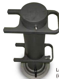
Low-frequency tube (internal diameter 100 mm)
