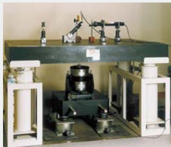
Absolute calibration setup for vibration accelerometers
