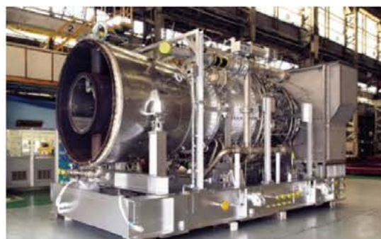
Figure 9 H-25 series gas turbine
