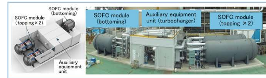
Figure 6 External view of 1 MW class half module demonstrator using MGT
