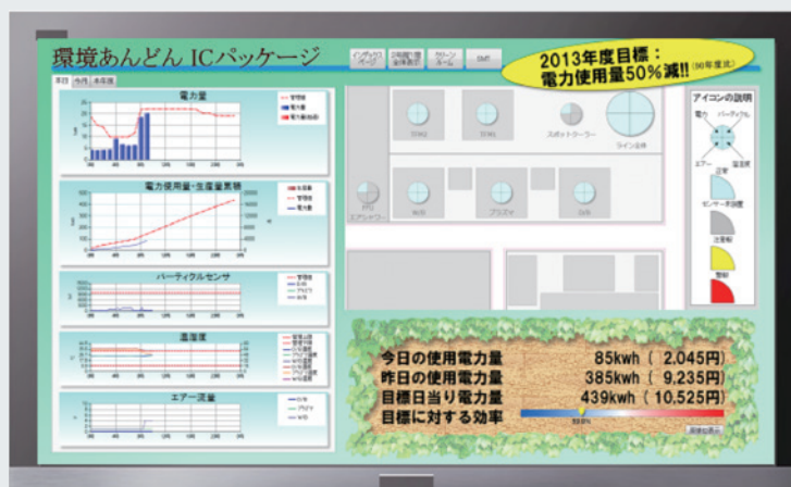
“Environmental ANDON” visualization system (PAT: Patent No. 4377353 (JP))
