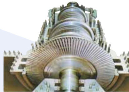
C type turbine (C9-R12-ER) with upper casing removed. (Typical example)
