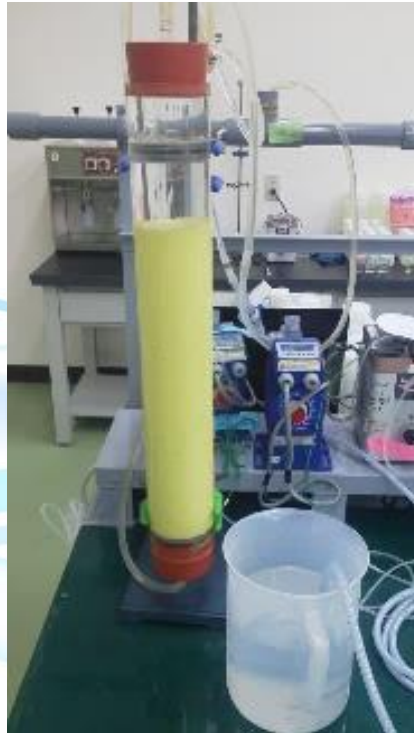
Column water flow test
