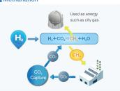
"Methanation" is a technology for synthesizing hydrocarbon compounds such as CH4, the main component of natural gas, from H2 and CO2,
