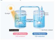
\*Artificial Photosynthesis" is a technology for synthesizing chemicals from water and CO<sub>2</sub> using solar
