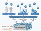
To reduce CO2 emissions, research is being conducted on "CO2 fixation": absorption and fixation of CO2 in
