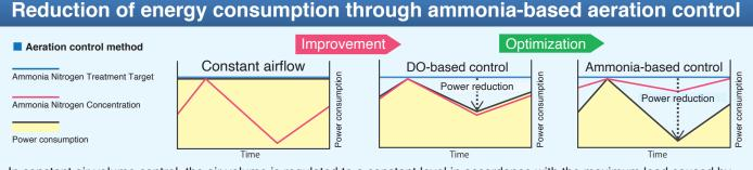
In constant air volume control, the air volume is regulated to a constant level in accordance with the maximum load caused by ammonia. As such, during periods of low load, excessive aeration occurs, resulting in wastage of power.
