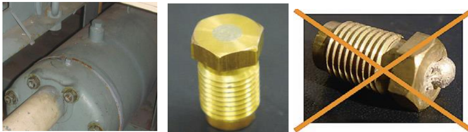
Deformation of a fusible plug
