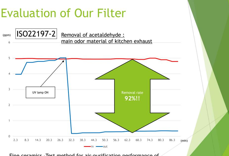
Fine ceramics -Test method for air-purification performance of semiconducting photocatalytic materials
