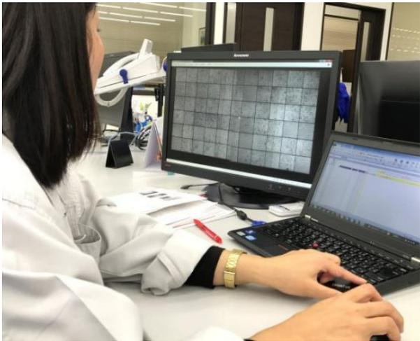
All of our solar modules are checked for cracks in the cells during manufacturing before being supplied.
