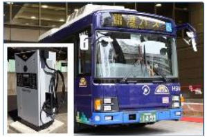
EV bus and charging station
