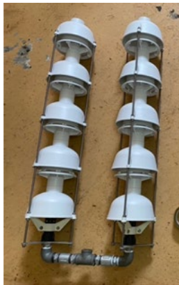
Liquid Film Aerator (The photo shows a 5-tube type)
