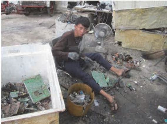
1) Hand dismantling of e-waste (no pollution control)
