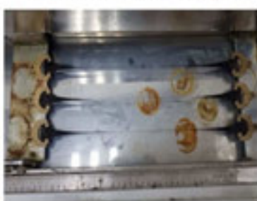
Figure 3.5 The early Failed of Ductility Test
