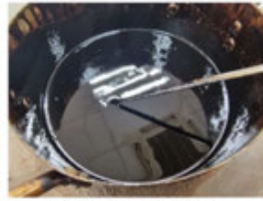
Figure 3. 3 Bitumen when mix with plastic for 12hours
