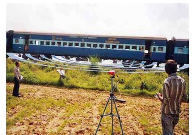
Monitoring unit railway noise level for Environmental and Social Impact Assessment for Dedicated Freight Corridor Project, India
