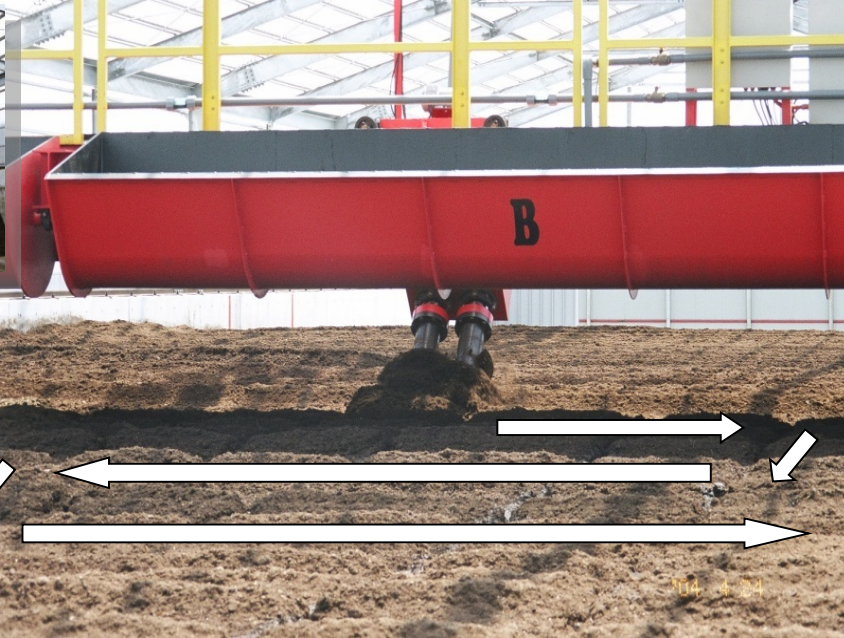
Movement of stirring screw by crank motion.
