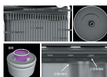
Example of Lithium-Ion Battery Internal Observation
