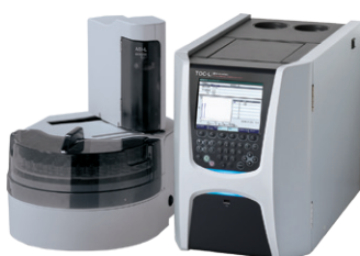
TOC (Total Organic Carbon) Analyzer
