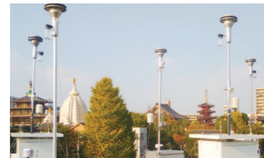
Parallel test of PM2.5 continuous measurement equipments
