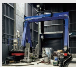
Largest construction 3D printer in Japan
