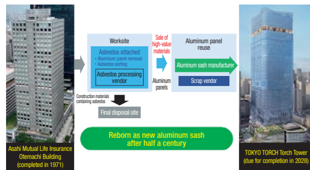
Flow for reusing aluminum panels
