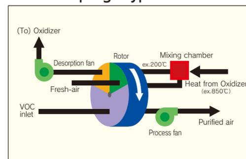
Note: Please note that use of mixing air with combustion gas will cause deterioration depending on type of inlet VOCs.
