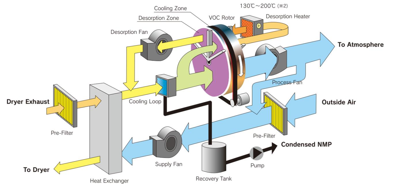
〈Basic NMP Recovery System diagram〉
