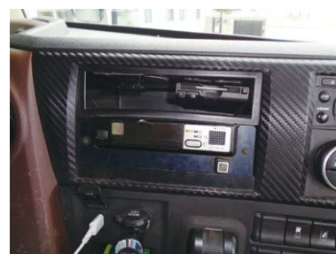
Improved fuel efficiency through the use of digital tachographs
