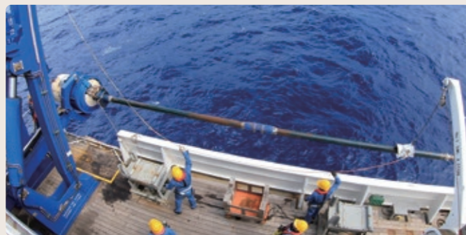
Giant Piston Corer (GPC) sampling sea floor sediments
