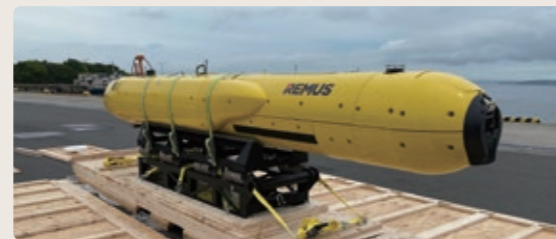
Autonomous Underwater Vehicle (AUV) capable of doing exploration down to 6,000m
