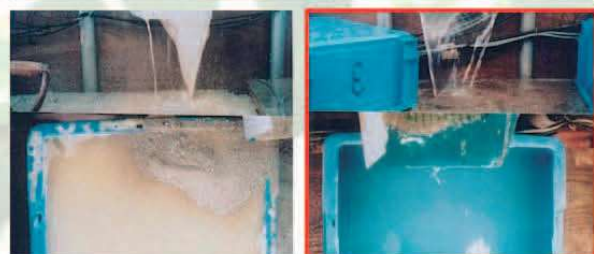
Conventional mat Takino Filter (Comparison of runoff after 10 min. of 100mm/hour rainfall)
