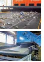
Our company aims to contribute to a low-carbon society and improve the recycling rate, so we have introduced an optical sorting machine and finely sorted, making it possible to increase the amount of raw materials for RPF.
