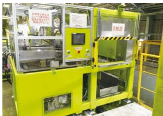
エアコン室内機簡易解体装置 Air conditioner indoor unit simple dismantling device
