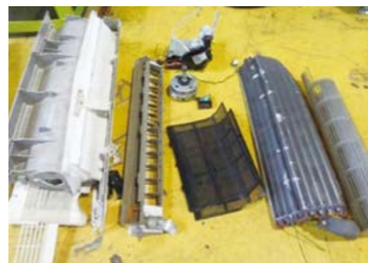
分解・仕分け後の室内機の状態 State of Air conditioner indoor unit after disassembly and sorting
